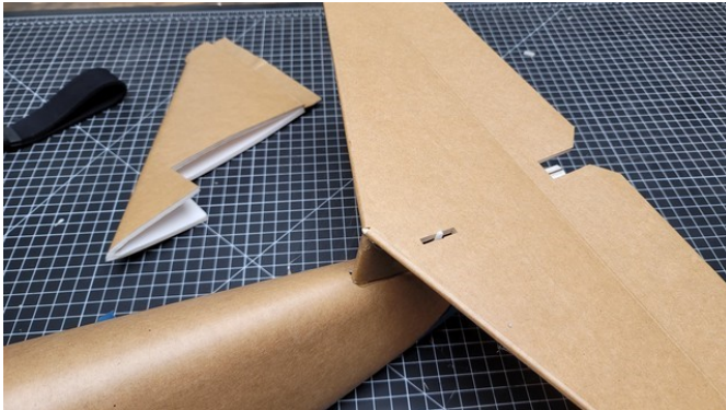
Glue horizontal stabilizer in place.
