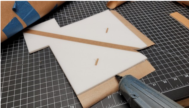
Add a bead of glue to edge foam as shown.
