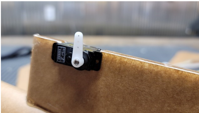
Install servo arm
