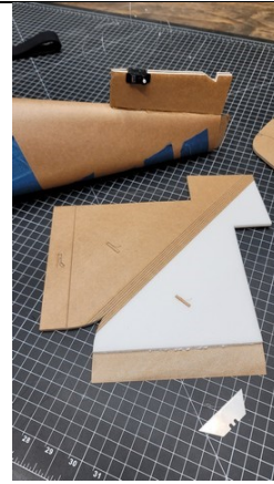
Glue small section of vertical stabilizer in place as shown. Follow symbol mapping instructions on vertical stabilizer.
