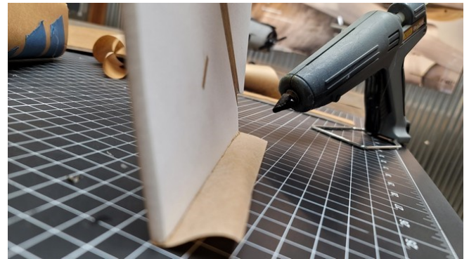
Stand foam on edge and allow glue to cool.
