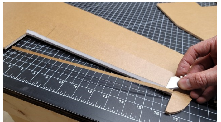
Add bevel along aileron. Reinforce hinge with light layer of glue. Make sure and wipe away all excess glue using foam scarp.
