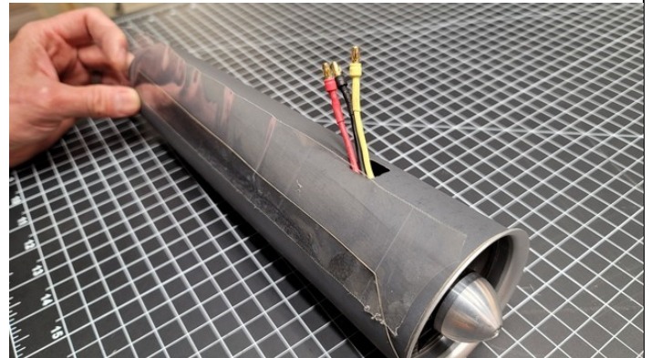
Run clear tape over seam.
