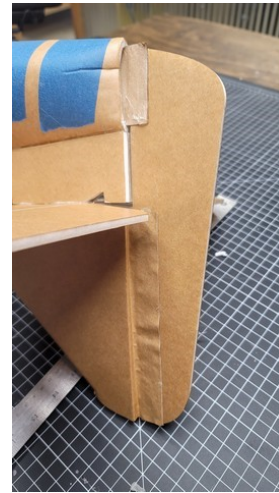
Glue on of the rudders in place as shown. (See spacing on next pic)
