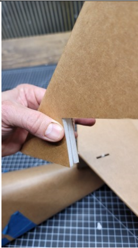
Pinch and hold till glue dries. Glue vertical stabilizer in place.
