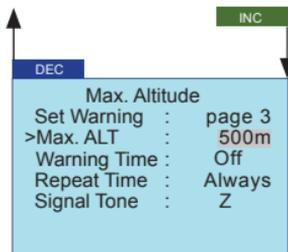
Maximum Altitude: Maximum altitude of the model during operation, warning threshold set between -500 and +3000 m (based on the starting altitude 0 m)
