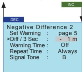
Sink rate/3 s (**Negative Difference 2**): Sink rate of the model per 3 sec. in Meter, warning threshold set between -50 and 0 m (based on the starting altitude 0 m)
