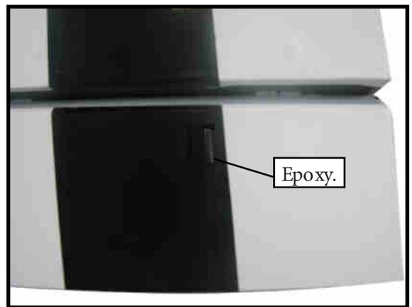
**INSTALL ELEVATOR CONTROL HORN.**
