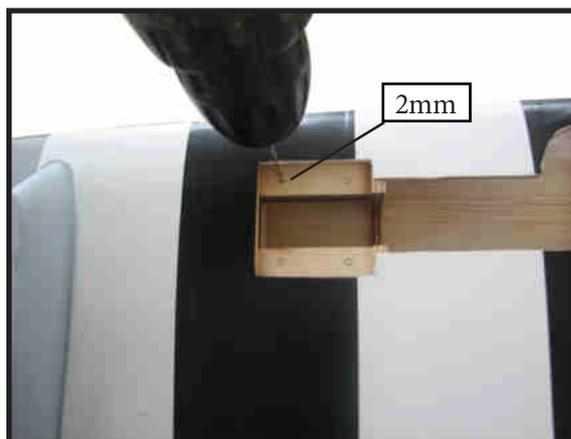
**INSTALLING RETRACTABLE LANDING GEAR.**
