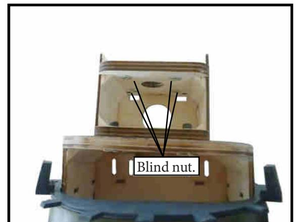
5) Attach the motor to the front of the electric motor box using four 4mm blind nut, four M3x15mm hex head bolts to secure the motor. Please see picture shown.
