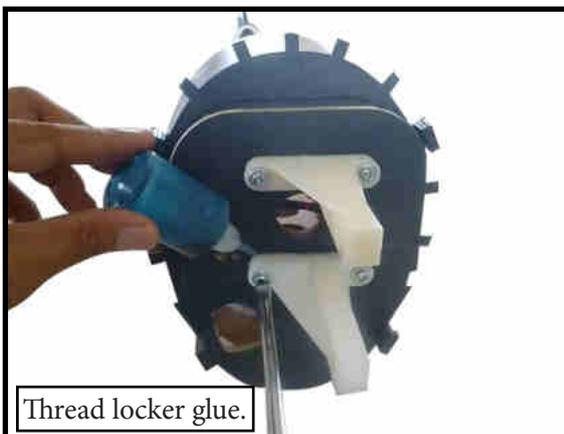
**MOUNTING THE ENGINE - 2 stroke.**
