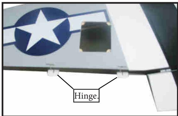
3) Slide the wing panel on the aileron until there is only a slight gap. The hinge is now centered on the wing panel and aileron. Remove the T-pins and snug the aileron against the wing panel. A gap of 1/64" or less should be maintained between the wing panel and aileron.
