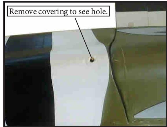
3) Tighten the antenna to the fuselage. The antenna is removable so you can install it at the flying field to prevent damage in transporting.
