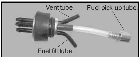
3) Carefully bend the second nylon tube up at a 45° angle. This tube is the vent tube.
