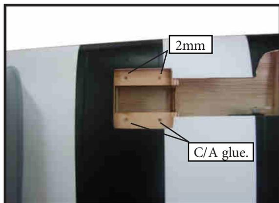
2) Install retractable landing gear at the Wing.
