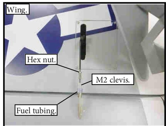
**INSTALLING THE FLAP PUSHROD.**
