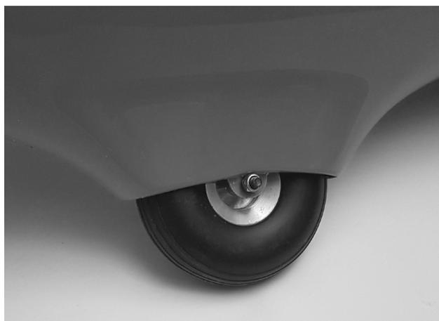
Now mount the main and tail wheel with Allen screws, nuts and spacers and pay attention to ease of movement.
