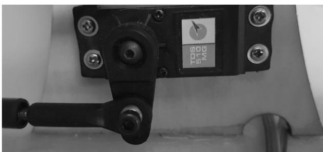
Now the linkage can also be hooked into the ball head of the servo and a mechanical length adjustment can be made.
