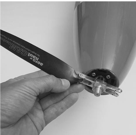
Thereafter, the propeller blades and the spinner cap are mounted on the middle section.
