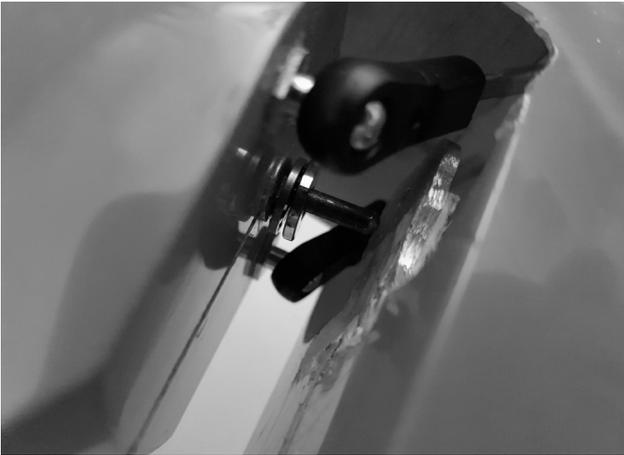
Now place the thrust bearing on the guide pin of the rudder and thread it into the receptacle of the fuselage. The ropes now hang into the fuselage. It has proven in this process, to put the fuselage 90 ° on the side.
