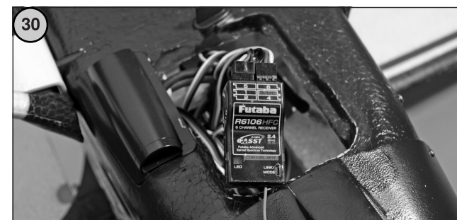
Fig. 30 Please refer to the radio control system instructions before tackling the next stage. - Assign the control functions by connecting the servos to the appropriate sockets at the receiver. - Connect the speed controller. - Install the receiver in the fuselage. - Deploy the receiver aerial(s) as recommended in the RC system instructions. - Stick two strips of Velcro tape (hook) in the battery well to secure the flight battery.
