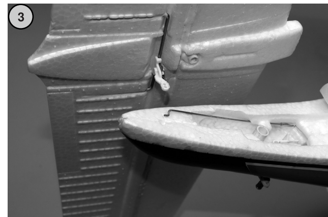
Fig. 3 - Draw the elevator pushrod back towards the tail.
