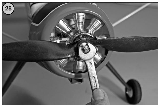
Fig. 28 - Fit the propeller, taper collet and spinner backplate on the motor shaft, leaving about 4 mm clearance between the dummy radial engine and the spinner backplate.
