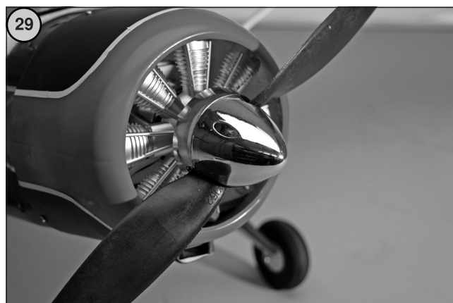
Fig. 29 - Fit the spinner cap and the retaining screws.
