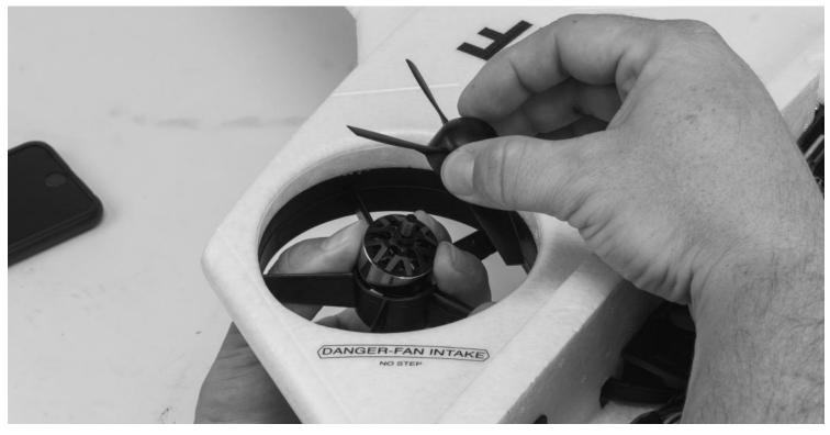
4. The rear motors use a traditional fan nut and spinner but do have different thread directions as with the front motors. Place the propeller over the appropriate motor, paying close attention to the direction (reference the diagram on the previous page). Place a fan washer over the fan on the motor shaft, followed by the fan nut. Tighten the nuts completely with an adjustable wrench.
