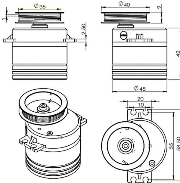
The Robbe FSW 220 Sail Winch is an extremely strong, robust and precise winch with a waterproof CNC aluminium housing (IP68), full metal gearbox and double ball bearing steel output gear designed for extreme loads and durability.
