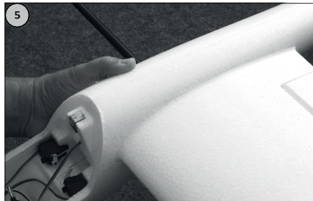
Pictures 4 and 5: Slide the wing into the recess in the fuselage. Carefully pull the connecting cable through the recess in the middle of the fuselage to the front of the fuselage.
