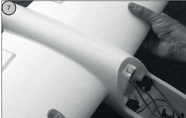
Picture 7: Now push the wings together completely.
