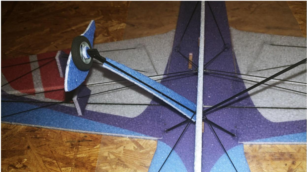
**Locate the EPP landing gear cover that will be placed over the carbon fiber landing gear leg. Test fit this piece, then glue it on over the carbon fiber using the pre-cut slot.**
