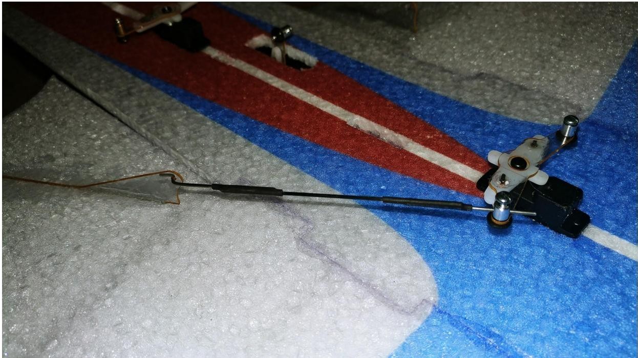
**Shown above is the entire aileron linkage assembly for one aileron. Notice the heat shrink over each glued end, as well as the straight end clamped into the mini EZ connector on the servo arm.**
