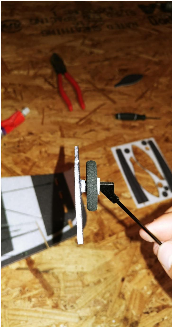
**Lastly, locate one of the wheel pants. You can place a bit of adhesive on the last foam collar before sliding the wheel pant on to the axle. If desired, you can place some adhesive on the outside of the wheel pant where the carbon fiber axle ends.**
