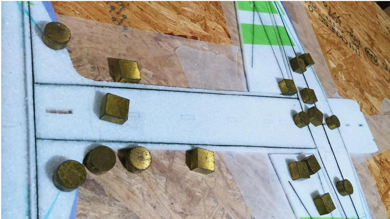
**The horizontal piece of the fuselage also uses flat carbon fiber spanning the entire length from the rear wing spar to the horizontal stab spar.**
