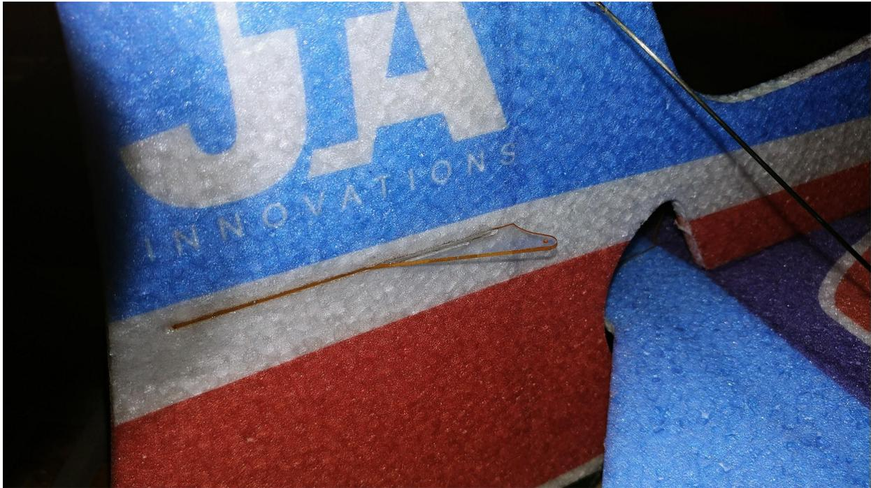
**You can now locate the final long control horn and glue it into the slot on the side of the rudder. This will be used for the rudder linkage that will be constructed in the same way as the one used for the elevator. Once again, the length for that linkage is 365mm. The guides for the rudder linkage will be glued into the top of the vertical fuselage.**
