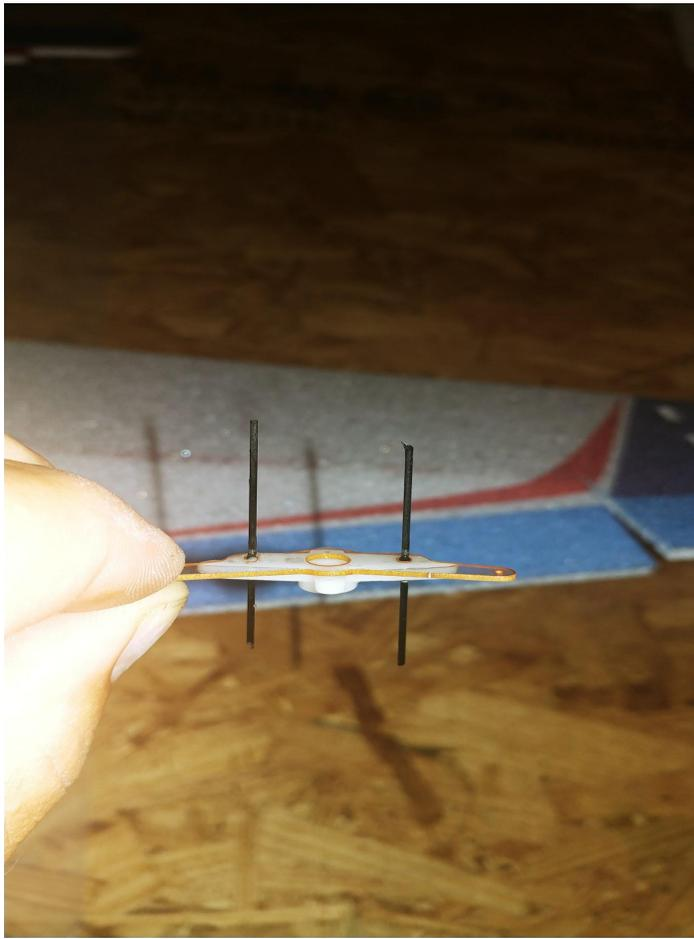
**You can now prepare your servo arms. Above is the provided double arm to be added on to the aileron servo arm that comes with the servo. Using the extension will provide the maximum amount of aileron throw. To join the two arms, use carbon fiber rods as shown above and glue them in through the holes lined up on each arm. It is important to use regular CA for this. You can then cut each rod down to shorten them.**
