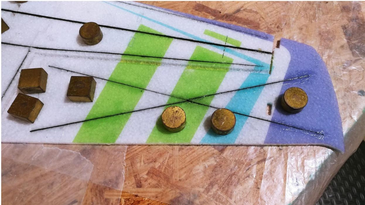
**As shown above, the aileron bracing is done using flat carbon fiber glued into the slots creating durability for the aileron. Please see the carbon fiber diagram for your airframe to determine which size carbon strips are to be used.**
