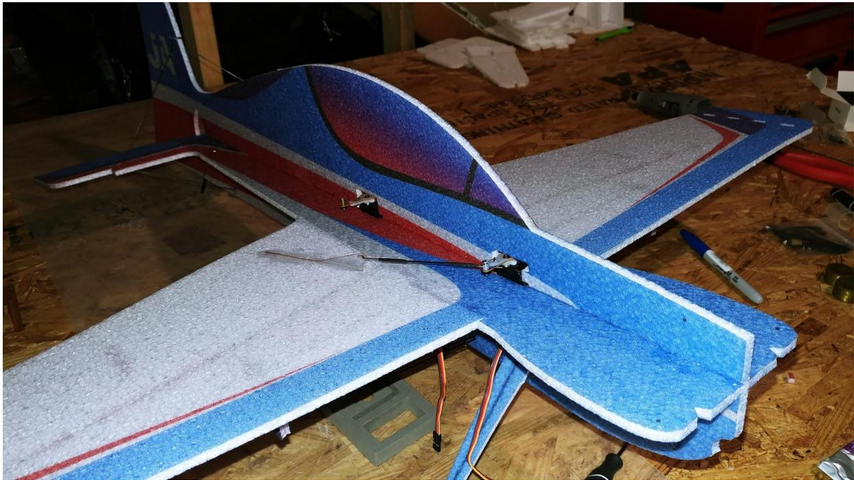
**Once the aileron and elevator linkages are set up, use the same process as glueing the bottom of the fuse to glue the top of the fuselage into place. Once again, it is important to keep this as straight as possible.**
