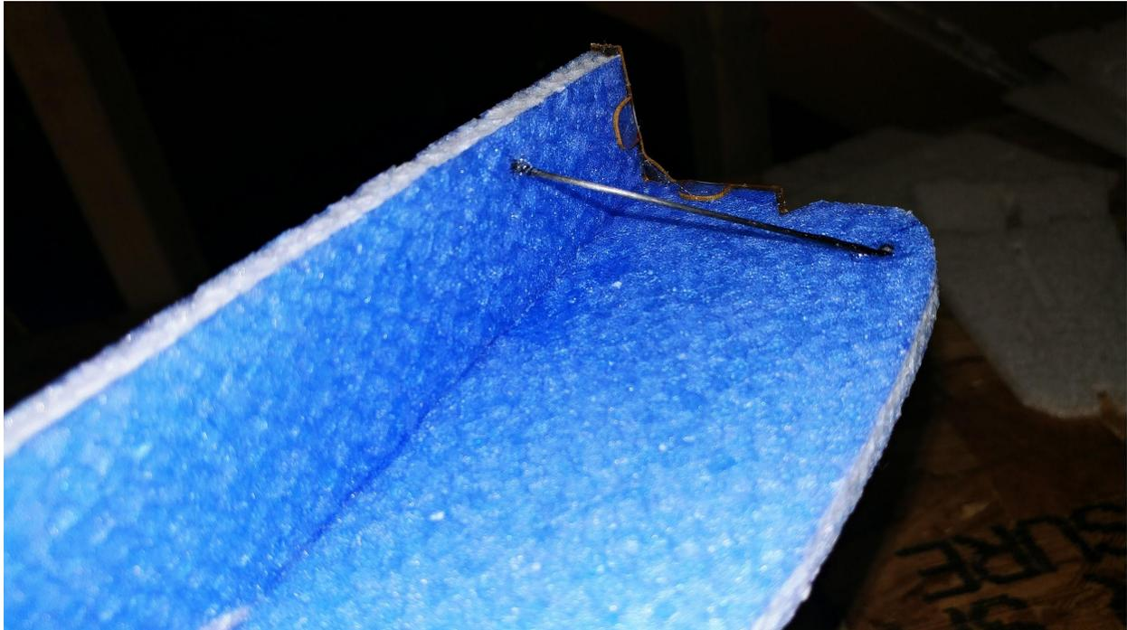
**The final piece used for carbon fiber bracing will be the rod used at the front of the airframe. Make sure that the fuselage is straight while these pieces are setting.**
