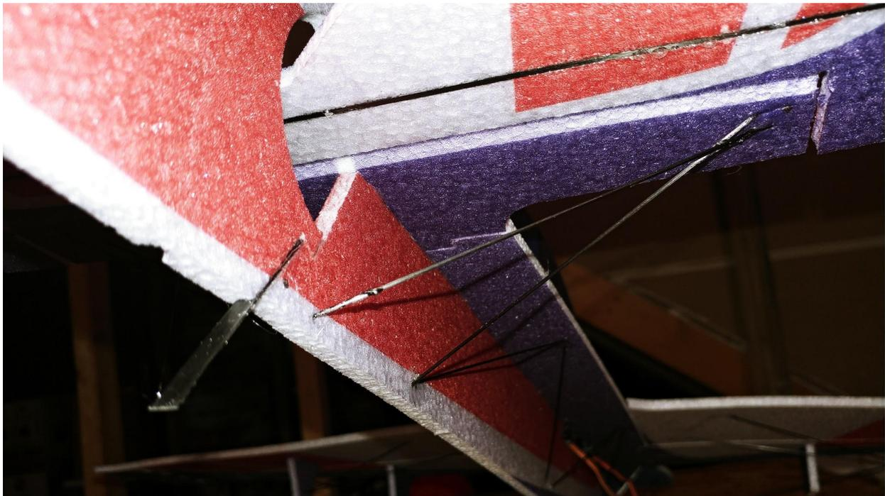
**Now that the top of the fuselage is glued in, you can glue the other rear carbon fiber rods to help strengthen the tail as shown above. They will be mounted from the bottom of the horizontal tail to the rear of the bottom vertical fuselage. Make sure they are glued in a location that allows for full down elevator throw.**
