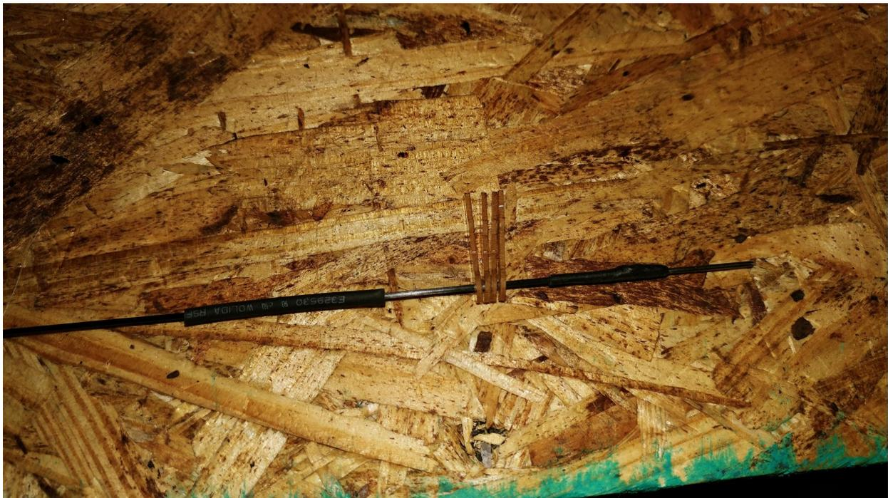
**Shown above is the elevator linkage. Notice how the 4 guides are slid over the linkage and the heatshrink is cut and slid on before the Z bend is glued. The rudder linkage will be done the same way later on. You will be able to tell where the guides will need to be glued in based on the slots in the fuselage.**
