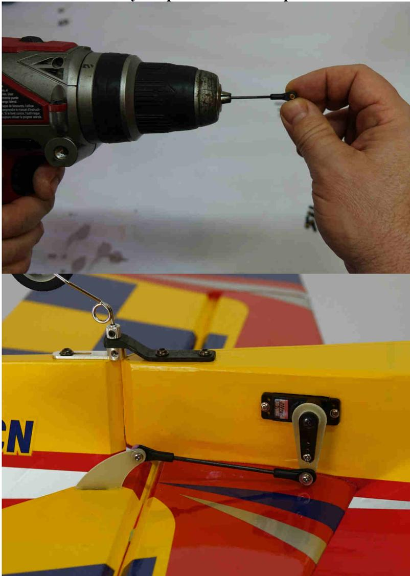
**18. Attach an 18" Extreme Flight 28AWG servo extension to the elevator servo lead and secure with heat shrink tubing or an Extreme Flight servo extension lock. Install the rudder servo and assemble the linkage as shown. The stock servo arm provides full rudder deflection.**
