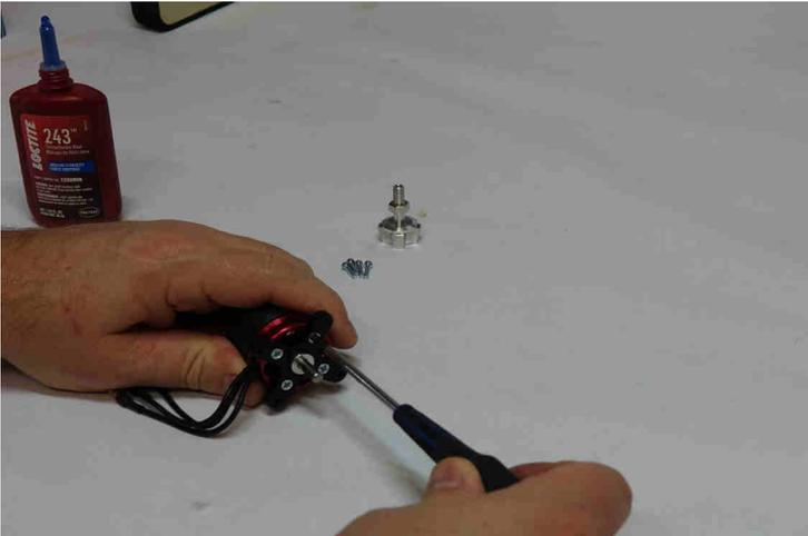
**8. Secure the prop adapter to the other side of the motor with the supplied socket head cap bolts. Remember to use blue thread lock compound on all bolts!**
