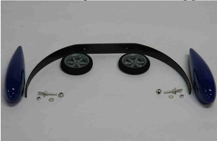
**2. Insert the threaded portion of the axle into the carbon fiber landing gear. Slide a washer onto the axle followed by a nylon insert lock nut. Do not tighten yet.**
