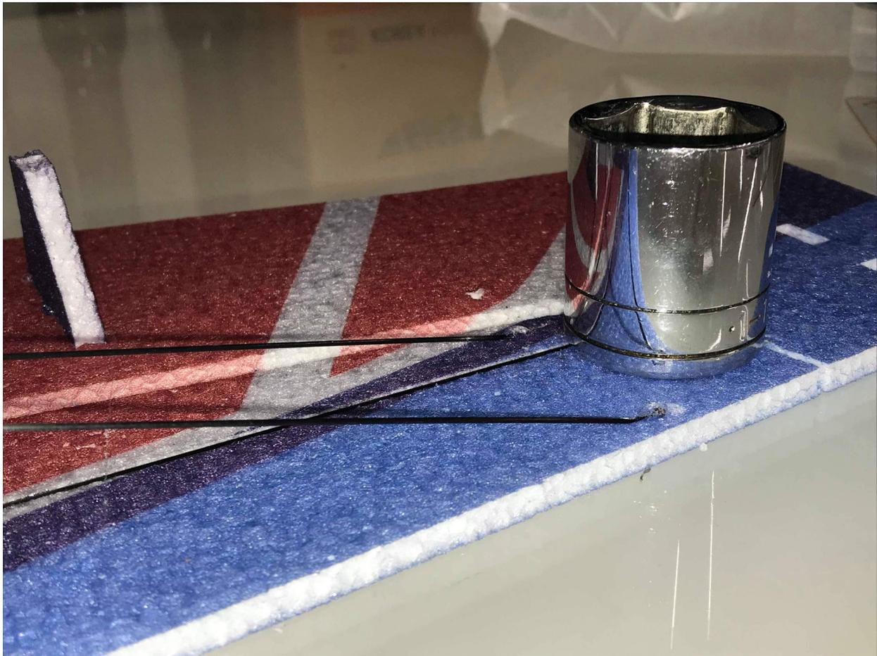
**Just like the aileron bracing, it is very important to use weight towards the wing tip while the carbon wing bracing is set up to keep the leading edge of the wing as straight as possible.**
