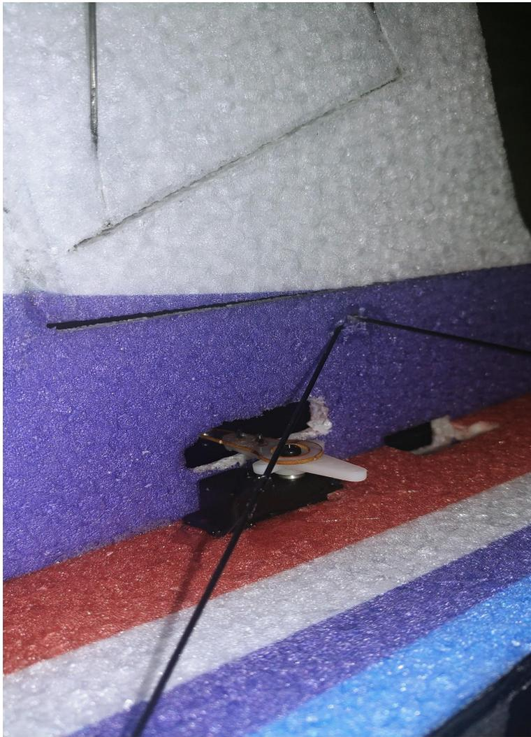
**Shown above is the glued in elevator servo. For the elevator, use the middle servo slot that is on the side of the fuselage. The arms used for the elevator and rudder servos are the singles. For both the elevator and rudder servos, face the output shaft towards the rear.**
