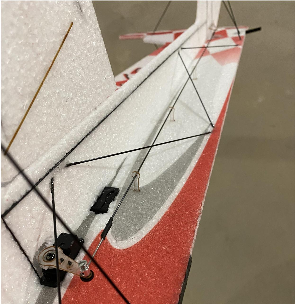
**Above is the finished elevator linkage setup with the guides glued into the fuselage and the elevator centered and clamped into the mini EZ connector. Also shown is the elevator control horn. It may be easier to glue the horn in after the linkage is assembled since the linkage is set up underneath the fuselage.**
