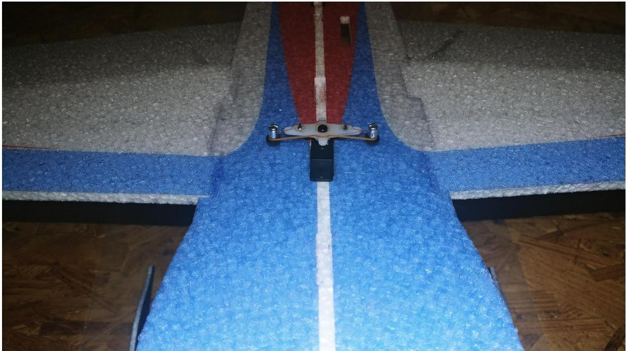
**After you electronically center your aileron servo by plugging it into your receiver and powering it on with zero sub trim and trim, you can glue it into the servo slot that is the most forward on the airframe with the output shaft facing rear. The aileron servo arm will be angled forward.**
