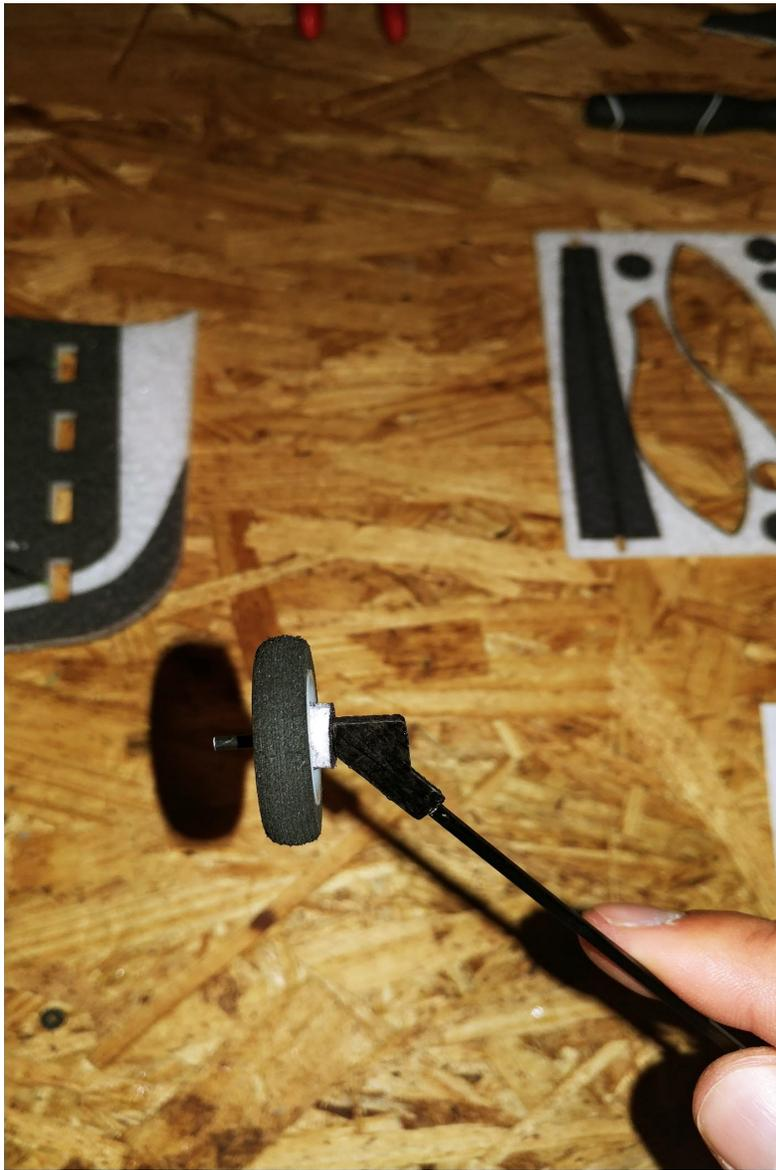
**Next, with no glue needed, slide one of the wheels on to the axle all the way up to the first foam collar. Make sure it is spinning freely.**
