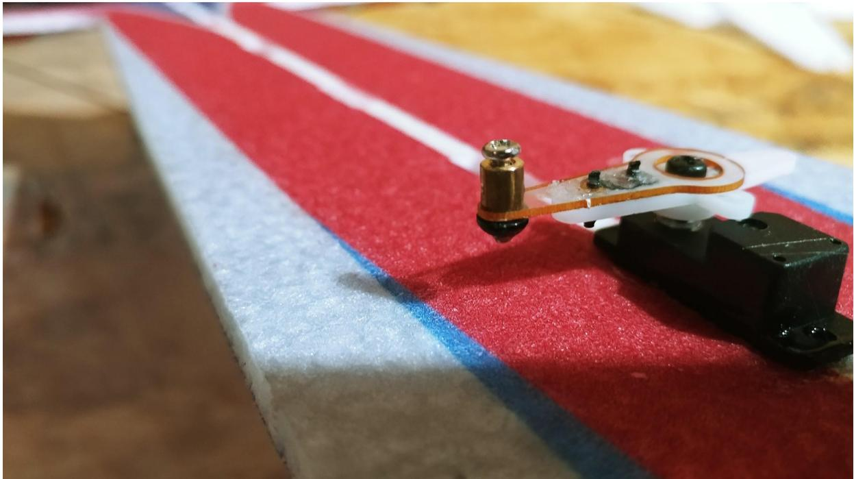
**Before placing the servo arm on the servo, locate the mini EZ connector.**
