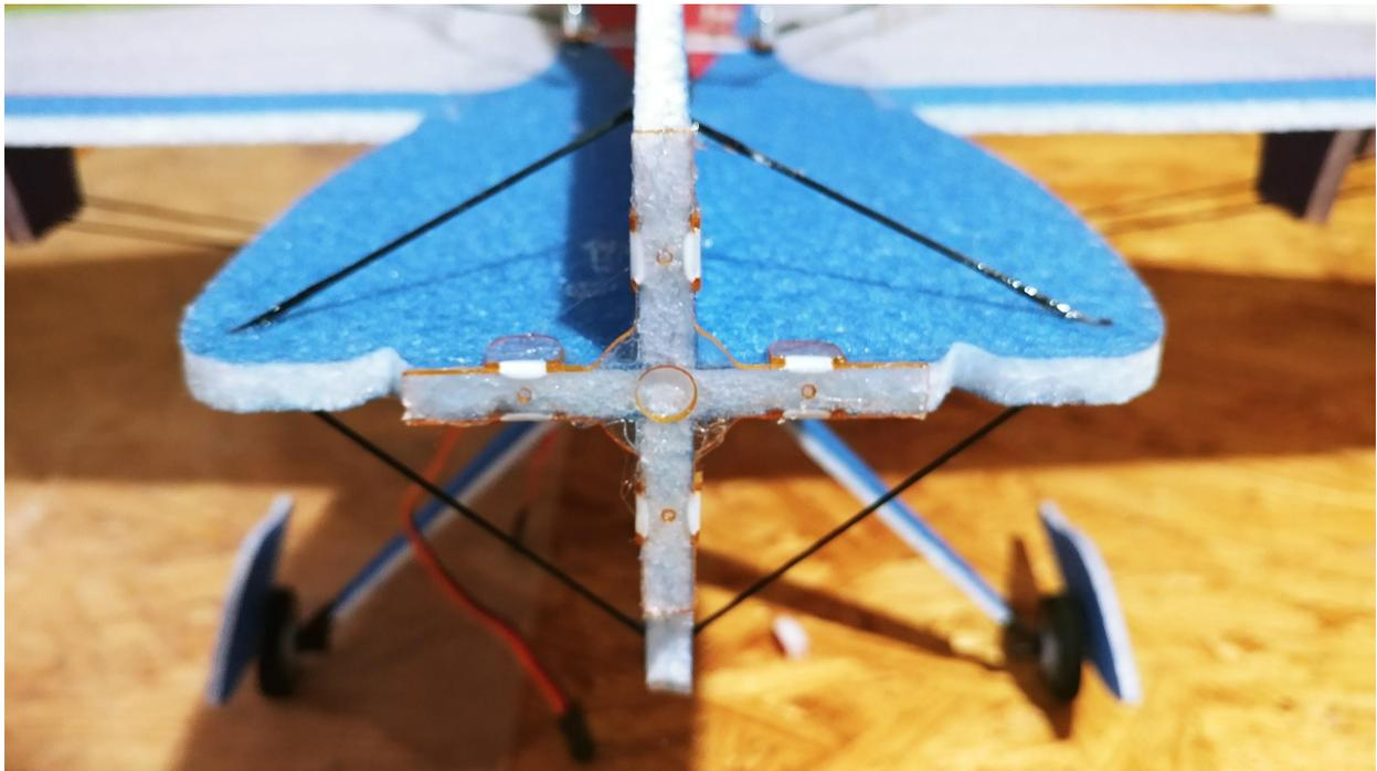
**Locate the motor mount as shown above. Test fit the motor mount to the front of the fuselage by bending the attached tabs 90 degrees and sliding it on without glue. Once test fitted, place adhesive on the inside of the motor mount covering every spot, then place again on the front of the fuselage making sure everything is flush and lined up correctly.**
