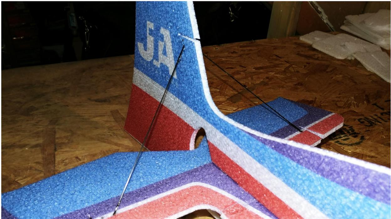
**Shown above is the carbon rod that will go on each side of the fuselage. It will be used to strengthen the horizontal stab and vertical stab.**
