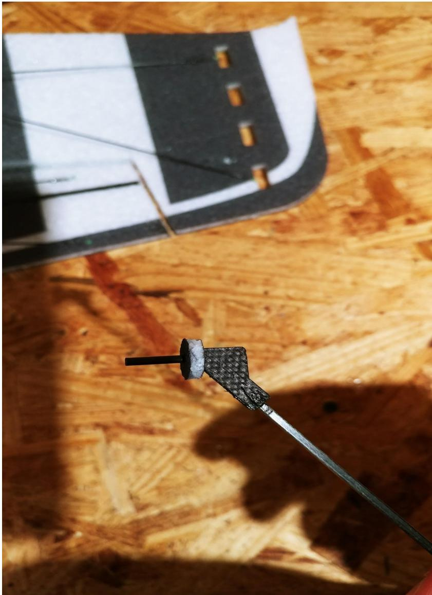
**Shown above is one of the carbon fiber landing gear legs that come pre-glued to the axle. The larger of the two EPP foam circular collars will slide on first. No need to apply glue to anything quite yet.**
