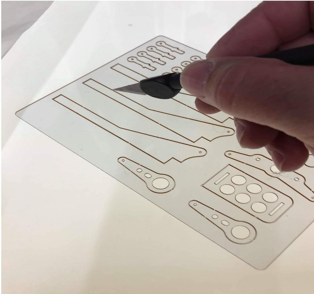
**Locate the control horns in the provided kit. You will find three longer horns and one shorter one. Two long ones will be used for the ailerons and one long horn for the rudder. The shorter one will be used on the elevator. You will notice a cutout on the bottom of the elevator horn that will fit over the elevator spar.**
