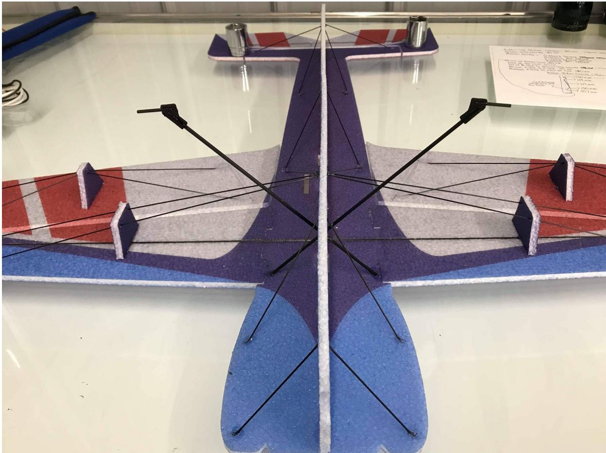
**Shown above are both landing gear legs in place. You will find the slots cut in the side of the bottom of the fuselage to slide each landing gear leg into. Make sure that the bottom of each leg is placed to where the airplane will sit level on the ground. Also shown are the first two carbon braces on the front of each side of the bottom of the fuselage.**
