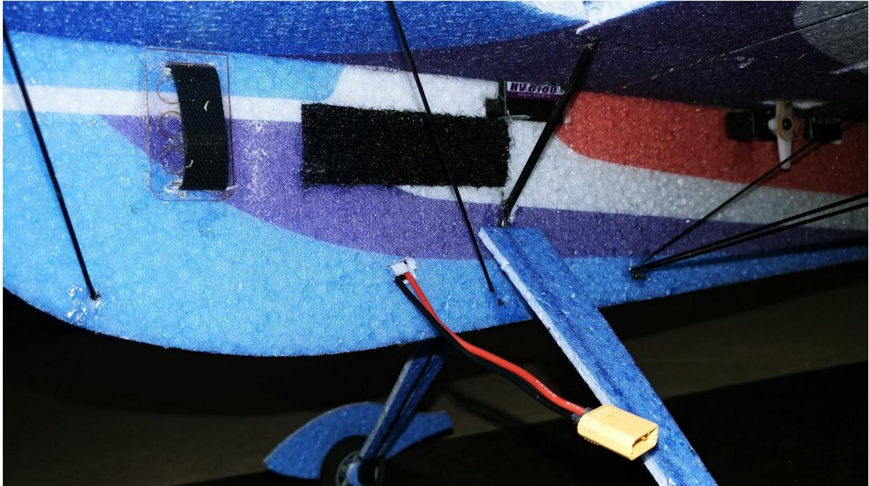
**The center of gravity and battery placement will depend on equipment used and personal flying preferences. The long piece of velcro mounted above is the location of the battery for this setup. To save space on the other side of the fuselage, the battery connector is put through to the opposite side of the ESC and receiver.**
