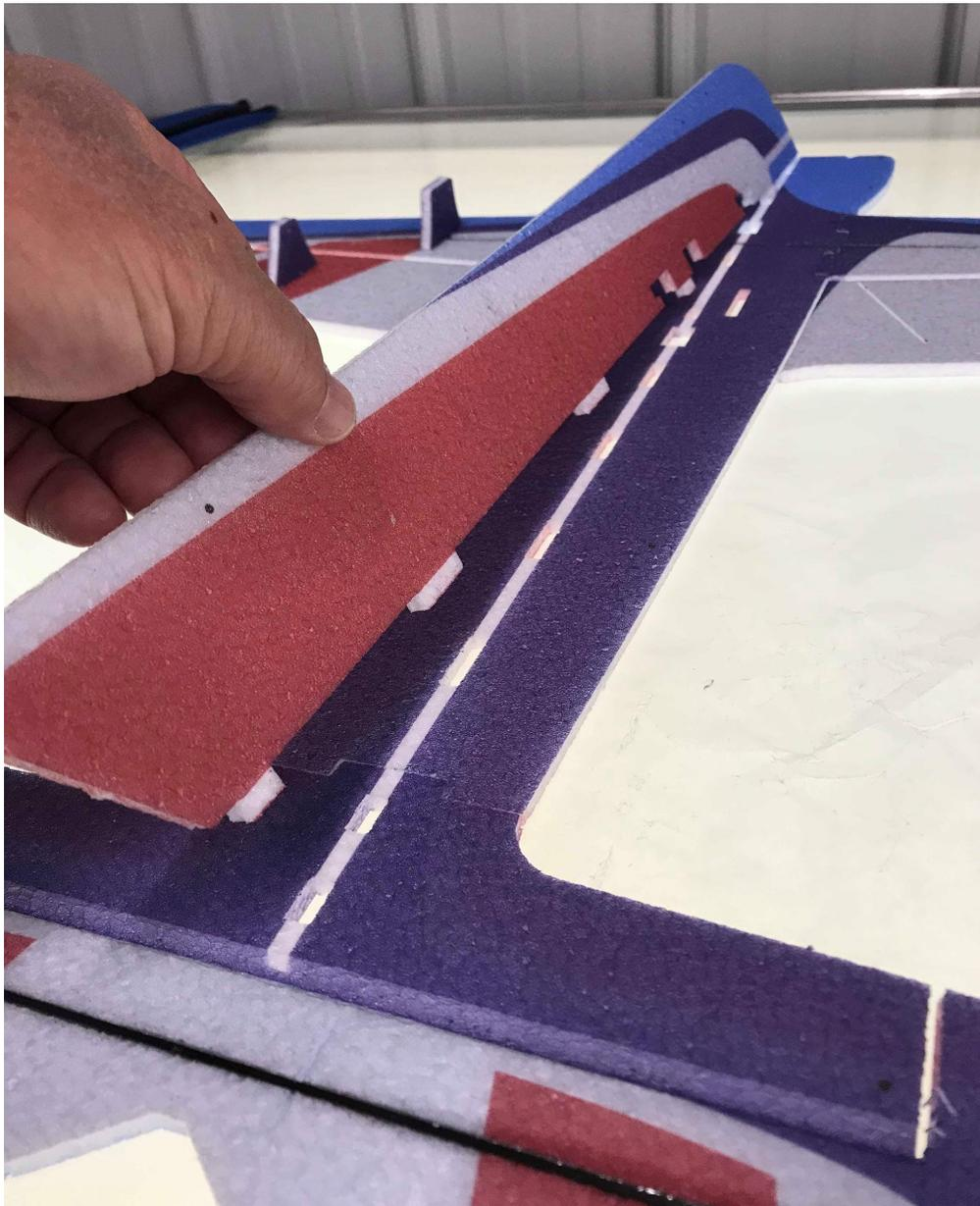
**You can now prepare the bottom half of the fuselage. Test fit this into each slot as shown above before gluing.**
