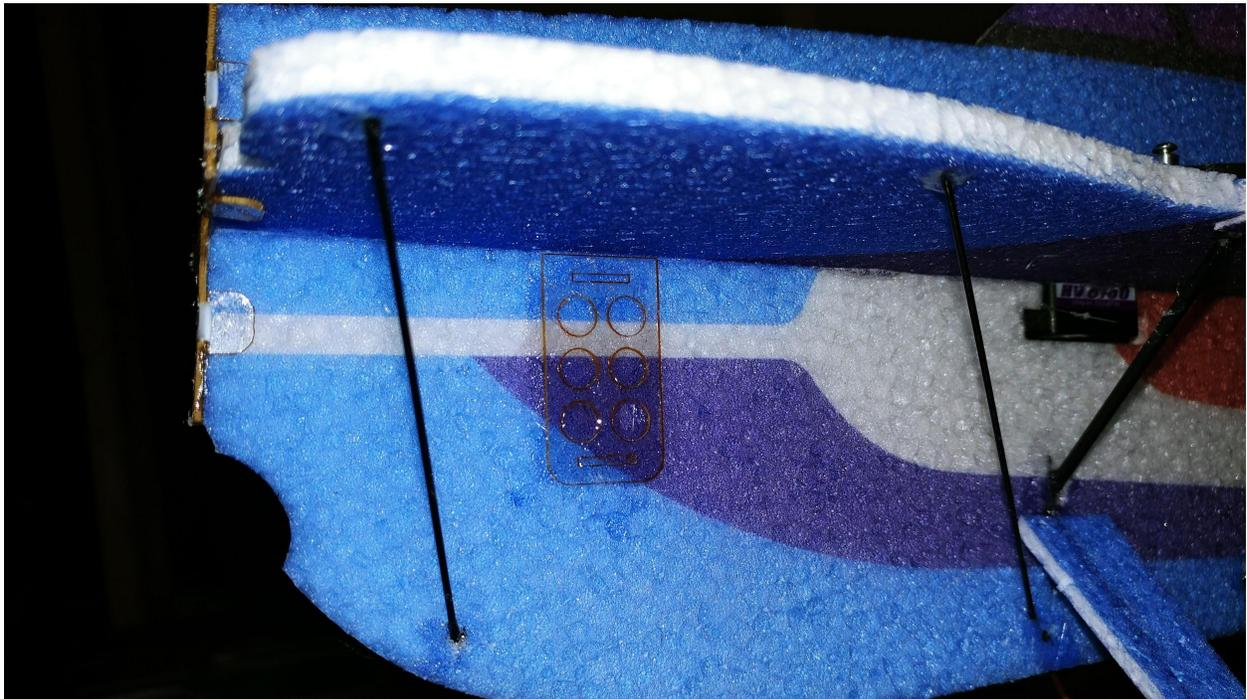
**Notice above the plate glued onto the side of the fuselage. This can be used to mount the electronic speed controller on the other side of the fuselage. The two cutouts on the top and bottom of the plate is where the provided velcro strap will slide through.**
