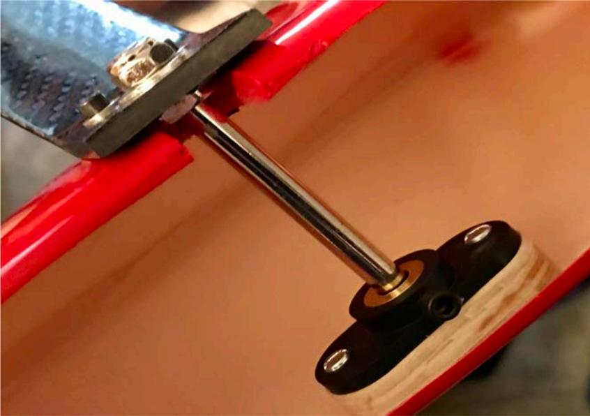
**16. Remove the wheel pants and secure the wheel to the axle with the provided wheel collars. We highly recommend that you file a flat spot on the axle for the wheel collar set screws to seat against.**
