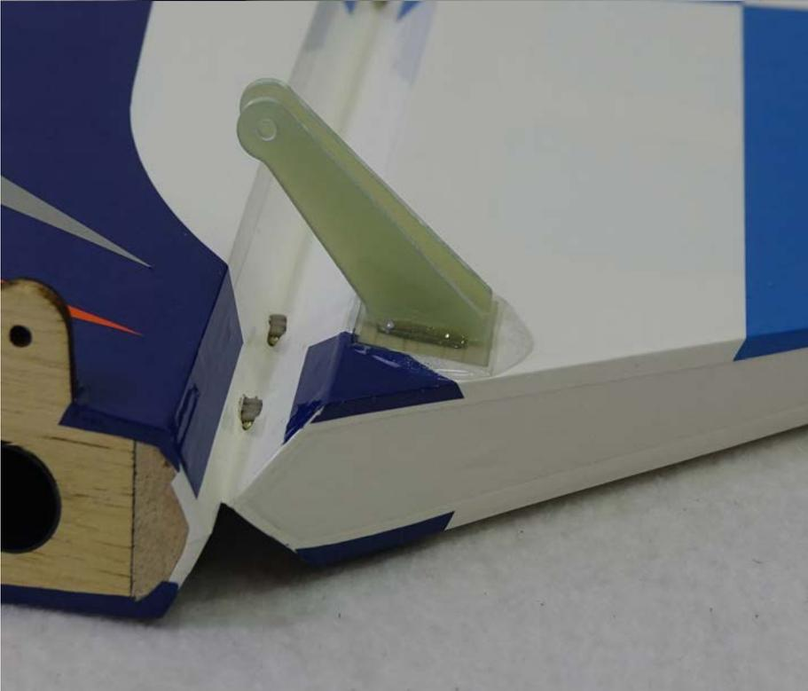
**8. Wipe away the excess epoxy with a paper towel soaked in denatured alcohol, making sure to do a good job of cleaning the area. Insert a bolt 3mm bolt and ball link into position and confirm proper alignment before the epoxy sets.**
