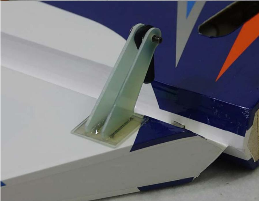
**9. Repeat this process for the other stab half, the aileron control horns and the rudder control horns.**
