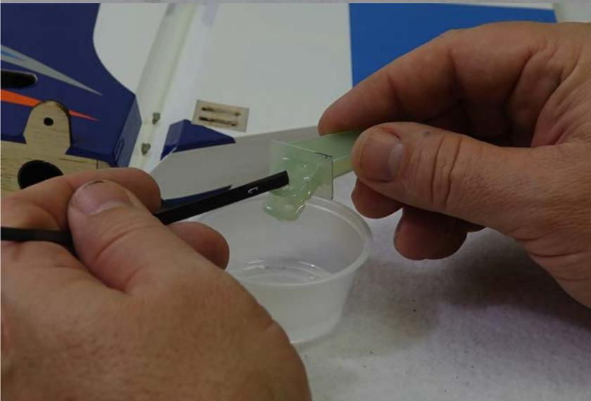
**7. Insert the control horns into the slots and ensure that the horns are properly seated against the base plate and the base plate is flush against the control surface.**
