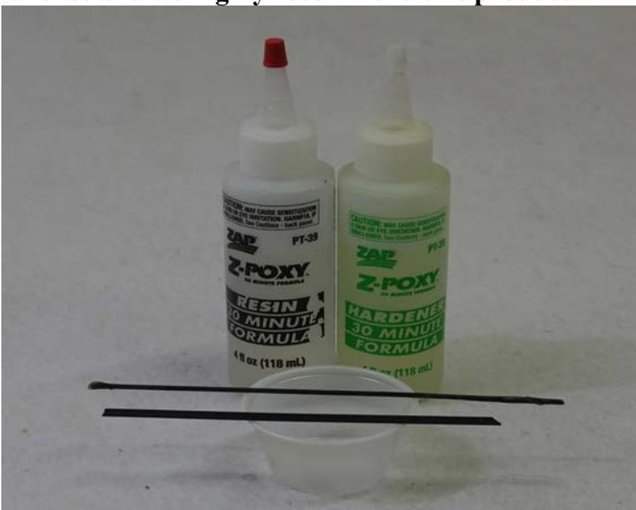
**5. Mix a generous batch of epoxy being careful to use equal parts resin and hardener.**
