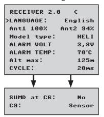
The receiver setup menu appears in the "Telemetry" menu under SETTINGS / DISPLAYS or if you are using a SMART-BOX under SETTING & DATAVIEW. How to access this menu is described in the operating instructions supplied with your transmitter or Smart-Box.
