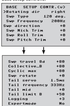
When a value is activated in the basic setting control, the gyro control and partly the control are deactivated! Therefore, settings must not be carried out in the air, but must be carried out on the ground without speed!
