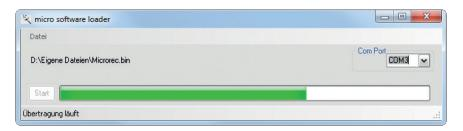
The progress bar shows that the transfer is running normally. The receiver LED lights up red during this process and flashes once the transfer is completed.
