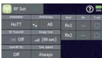
If the bind was successful you will notice in the Rx column of the transmitter the number of receiver channels for example R6, R12 with a highlighted blue background and the LED on the receiver will change its color or state.
