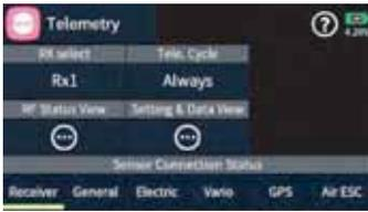
The telemetry connection between the transmitter and receiver takes place via the return channel of the HoTT receiver defined as the main receiver. If more than one receiver is bound to a model memory, the return channel will be by default the last bound receiver. This assignment can be changed in the submenu "RF Set" in the base menu or at the special "Telemetry" menu.
