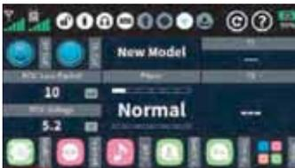
The main display is designed around user editable display widgets that can be changed and adapted to your own personal needs. There are in total six editable decks that can be accessed with the left/right arrow keys on the radio.
