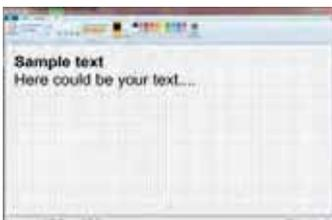
Pages should be in landscape format sized at 440 x 232 pixels. After creating any type of content, save it in "BMP image" format under "Save as" with the file type "24-bit bitmap (\* .bmp; \* . Dib)". In Paint 3D, under "Save as file" select "Others" and then as storage format "2D-Bitmap (\* . bmp)". The storage location is the corresponding subdirectory of the "Help" directory of the transmitter and the file name is the next free three-digit number.
