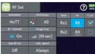
Up to two receivers can be bound to each model memory in the submenu "RF Set". However, a telemetry connection can only be established to one of these four receivers. The standard telemetry receiver is always the last one bound.
