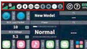
The operation of the display is analogous to the operation of other touch-sensitive displays, by tapping the desired option with the fingertip or with a pen suitable for capacitive displays. The only exceptions are the status indicators of the six freely configurable main displays, which are outlined in red on the top left.
