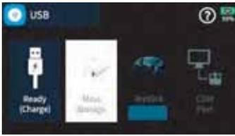
Firmware updates for the transmitter can be done wireless over a WiFi network or via the back of the radio using the micro USB port. When the transmitter is connected to a PC the USB menu is automatically shown.
