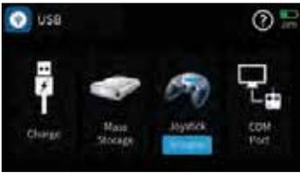
After connecting the transmitter to a USB power source, the display switches to the display shown on the left.
