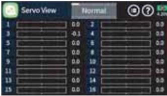
The Servo View monitor can be called upon at any time by pressing the servo monitor key on the right side of the radio.
