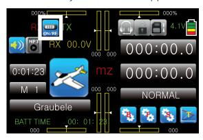
The red "RX" and green "TX" on the left and right of this switch symbol mean that the currently active model memory has once been linked to a *Graupner*-HoTT receiver but is presently not linked.
