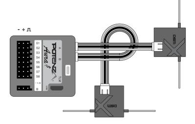
Note: It may be necessary to move the ESC lead to another open port (such as 'Port B') during the binding precedure. Be sure to return the ESC lead back to S1 after binding is complete.
