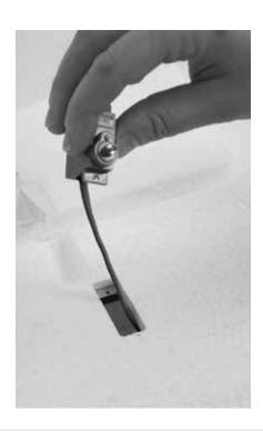
TIP: Plug a spare servo extension into the servo lead before removing to make it easier to install the lead of the servo when replaced.
