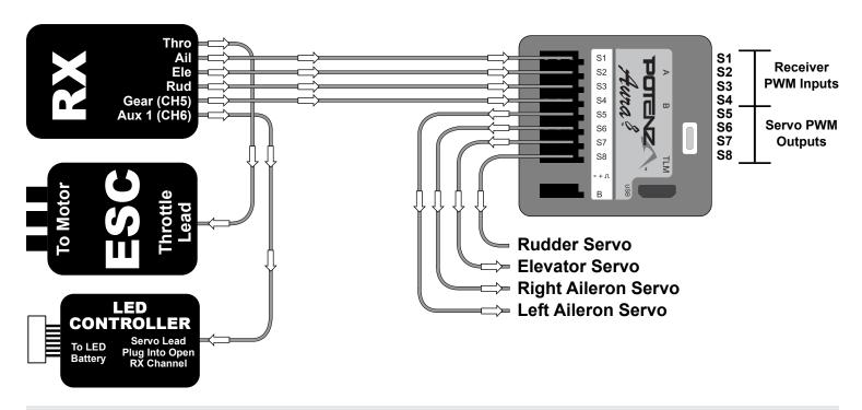
Note: The LEDs on the QQ Extra 300G2 Night Version are able to be turned on and off via a channel from your transmitter. For PWM users, simply plug the servo lead from the LED controller into any open channel on your receiver (such as CH6/AUX1), and assign that channel to a 2-position switch on your transmitter accordingly.
