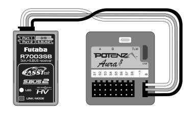
Note: If you are using Futaba S.Bus, be sure to use the proper S.Bus port in your receiver. DO NOT use the S.Bus 2 port, as it is not supported for use with the Aura 8. Refer to your manufacturer's instructions for proper S.Bus use.
