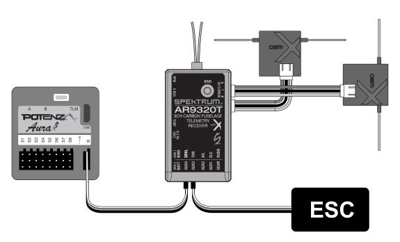
Note: When using Spektrum SRXL to connect to the Aura, always connect the remote receivers to the Spektrum receiver, NOT to the Aura.
